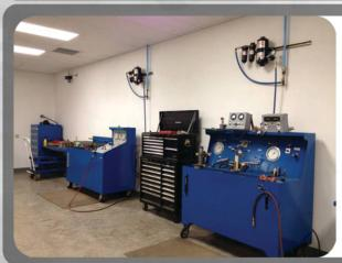
UME Inc. has developed test equipment to meet the high standards demanded by the mining industry. Every valve has documented test procedures that are followed stringently by the technicians. With 100% testing we insure that every valve meets all the requirements that it will give it a long productive lifecycle.
